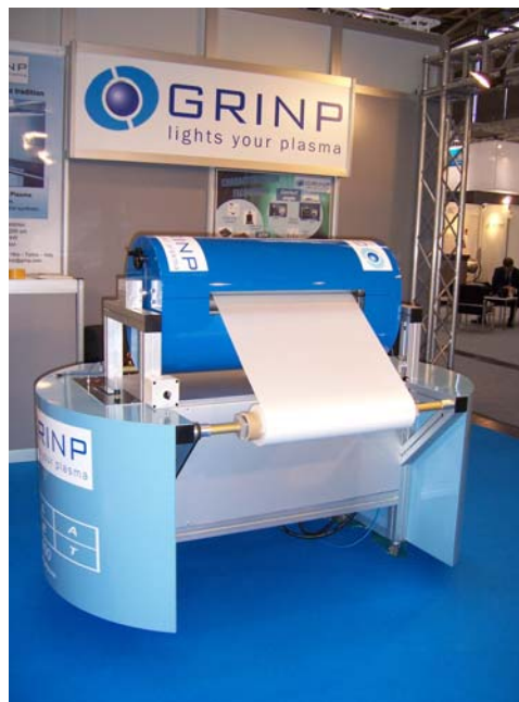
Figure 1. 60cm-wide APP machine for treatments of belts and tapes.
