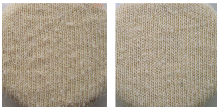
Figure 6. Knitted wool fabrics untreated (left, grade 1) and plasma coated (right, grade 2) at 5000 rubs.
