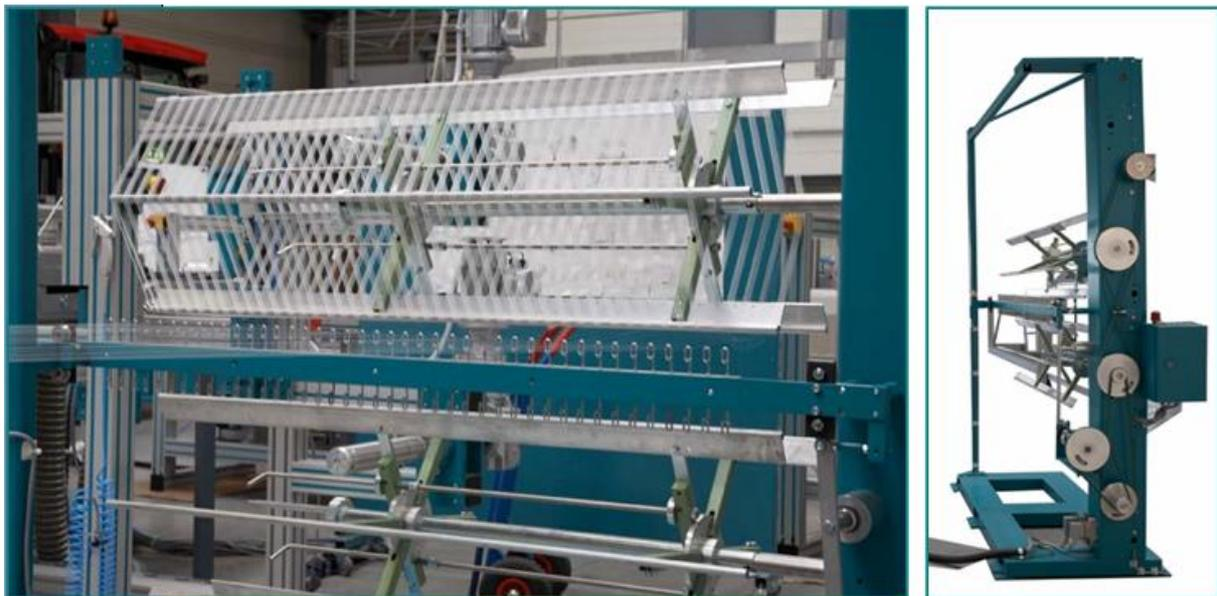
Picture 13: Winding-up coated filaments by a hank
