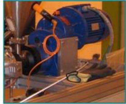
Picture 8: Coating by extrusion with hotmelts
