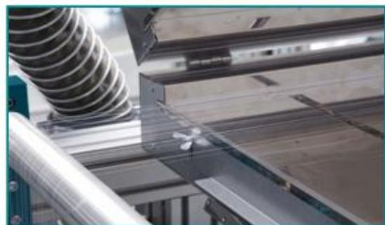
Picture 9: Drying with hot air
