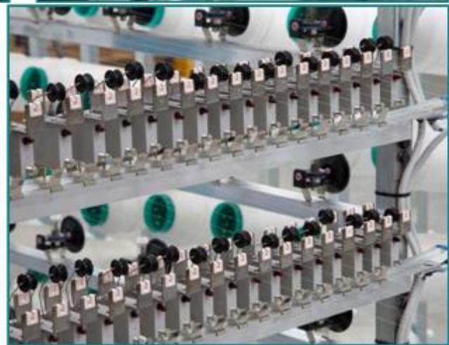
Picture 4: guiding by combs and ceramic eyes and rolls
