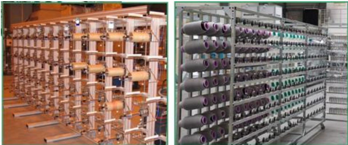
Picture 2: Creel in a filament coating machine
