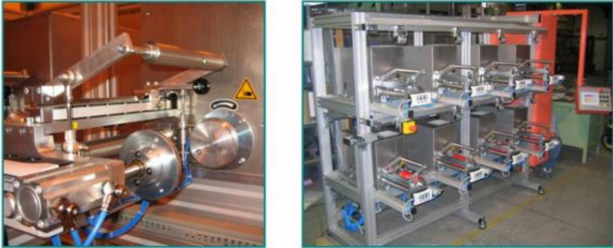
Picture 12: Winding on on single bobbin coil units or a creel
