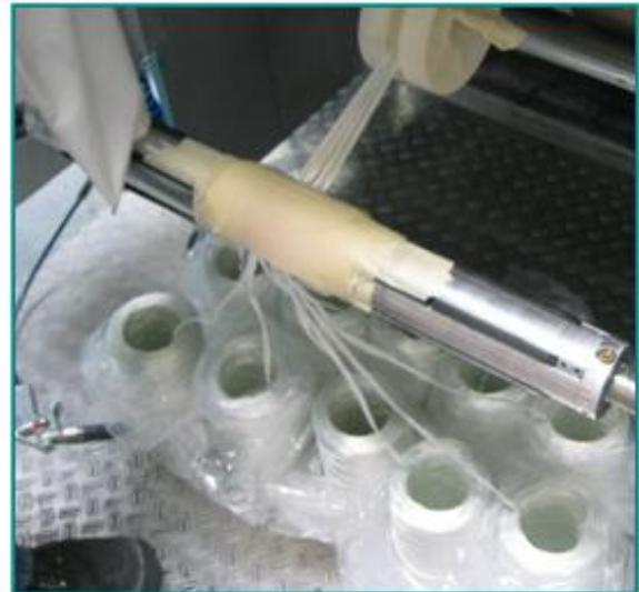
Picture 3: Winding off from bobbins
