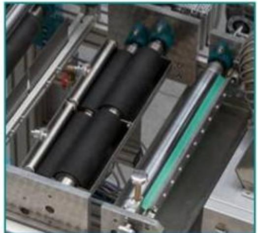
Picture 7: Coating with specialized two roller application systems
