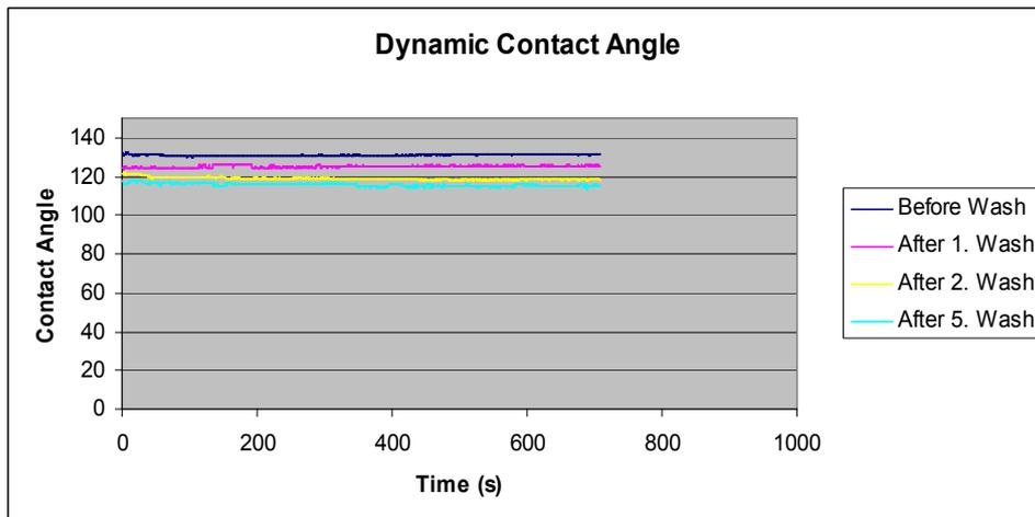
Graphic 11: Dynamic contact angle measurements of DBD treated fabrics finished by Baygard AFF 300 % (20 g/L).
