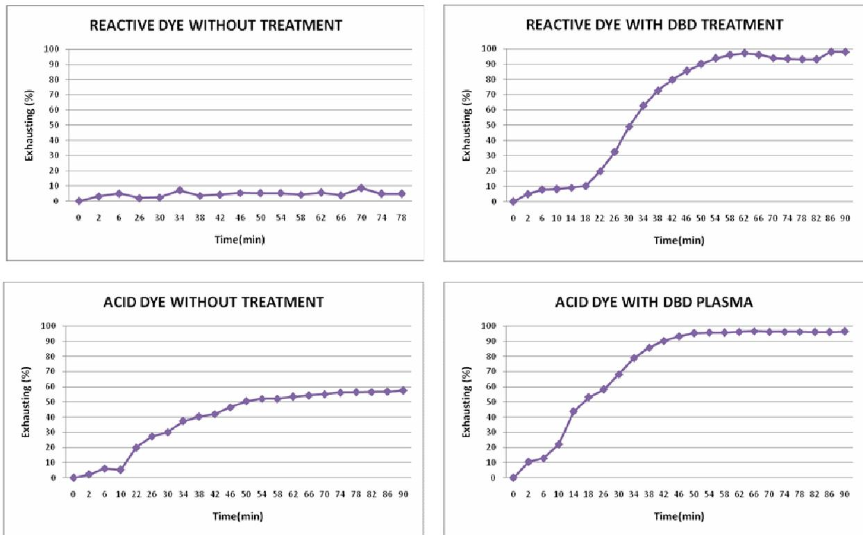
Graphic 7: Exhaustion of acid and reactive dyes in polyamide 6.6 with and without DBD plasma treatment.
