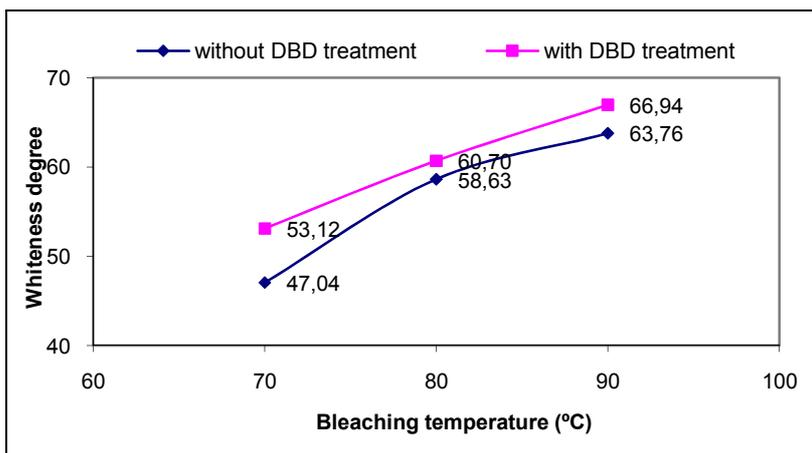
Long-bath bleaching process with hydrogen peroxide at the temperature of 70°C, 80°C and 90°C have been performed.
