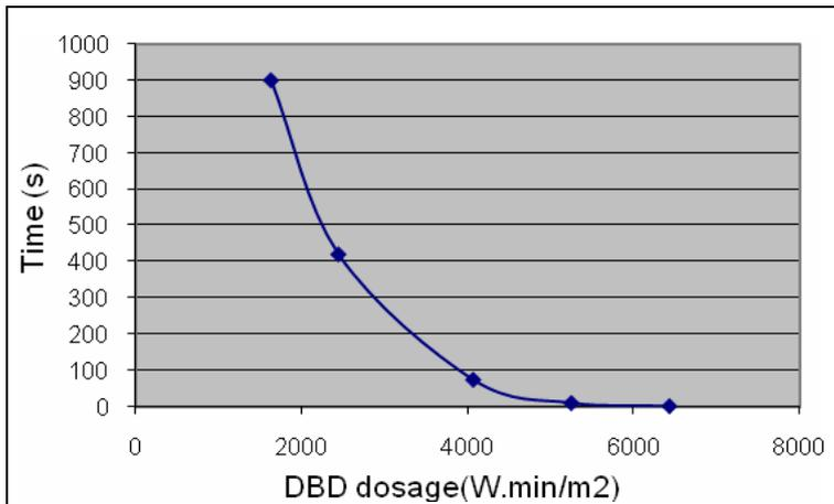
Graphic 2: Time for water drop absorption in raw cotton fibre versus DBD dosage
