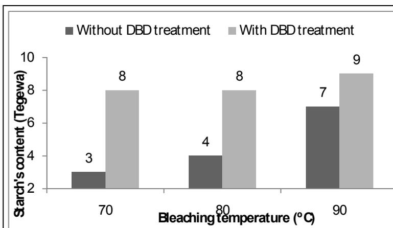
Graphic 5: Starch's content (TEGEWA scale) for different bleaching temperatures with and without DBD treatment
