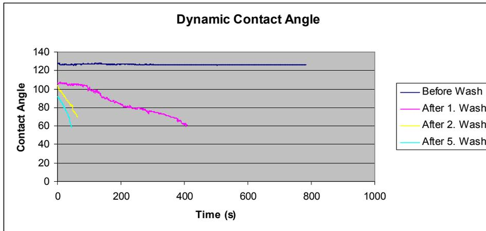
Graphic 10: Dynamics contact angle measurements of untreated fabrics finished by Baygard AFF 300 % (20 g/L)
