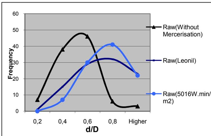
Graphic 3: Frequency analysis of d/D ratio (perpendicular axis of transversal cross-section) for mercerized and non mercerized raw cotton
