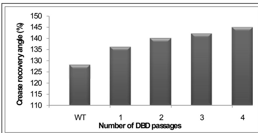
Graphic 8: Crease recovery angle for different DBD passages, after no-iron finishing with reticulation resins of low formaldehyde content
