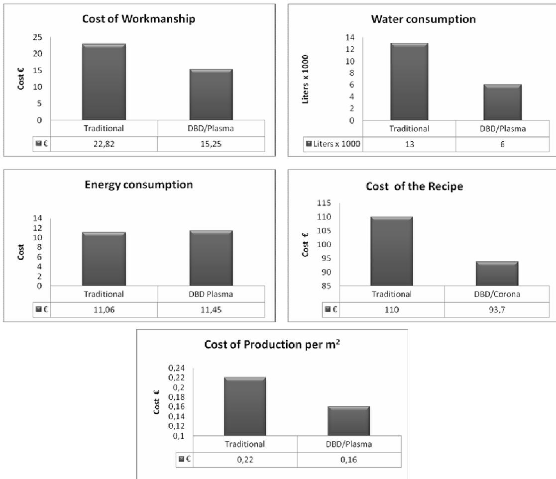
Graphic 1: Cost Comparison between traditional process and DBD Plasma process
