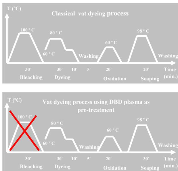
DBD plasma technology applied to vat dyeing enables a complete hydrophilization of raw cotton through oxidation of the hydrophobic layer, making cotton materials ready to be directly dyed, skipping the stages of preparation. The differences between conventional vat dyeing process and the process in which DBD is used, include the total annulation of preparation and a posterior half bleaching instead of the soaping used in classic vat dyeing.
