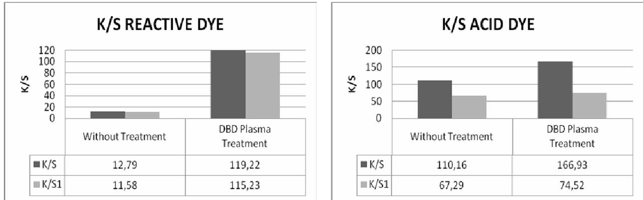
Graphic 6: K/S comparison results for polyamide 6.6 samples with and without DBD treatment. \*K/S1 – Values obtained after extracting treatment (solution 50% Urea; 100° C; time-30 minutes).
