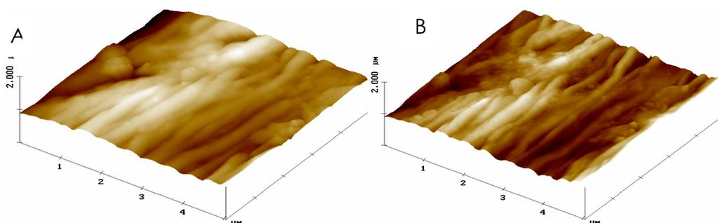
Figure 2: Images obtained with AFM of the cotton fibre before (A) and after (B) DBD plasmatic treatment
