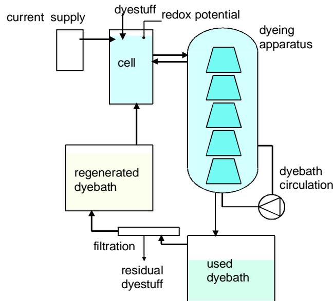
Figure 2. Scheme of the installation: Package dyeing apparatus, circulation through cell, regeneration of used dyebath by Nanofiltration
