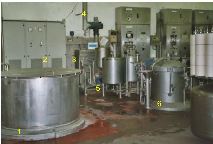
Figure 3. Installation of ECDVAT dyeing unit at Getzner Textil AG. 1 Storage tank, 2 cell current supply, 3 cell, 4 exhaust fan, 5 dye bath circulation, 6 dyeing apparatus
