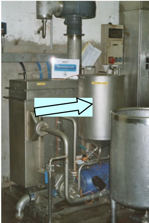
Figure 4. Electrolyser (the arrow indicates the flow of the dyebath through the cell)
