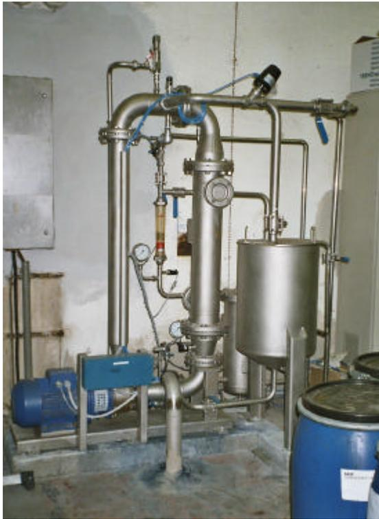
Figure 6. Full scale nanofiltration unit for dyebath regeneration
